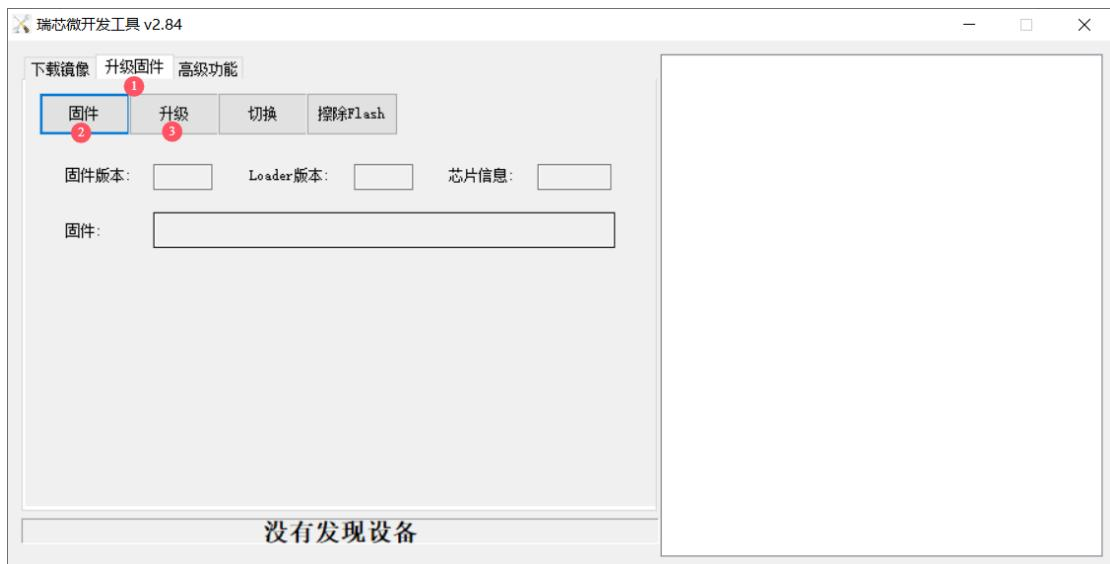
Partition Image Flashing: Extract RKDevTool\_Release.zip, double-click RKDevTool.exe file, to select the option box ->The blank area is loading the partition firmware-> Execute
