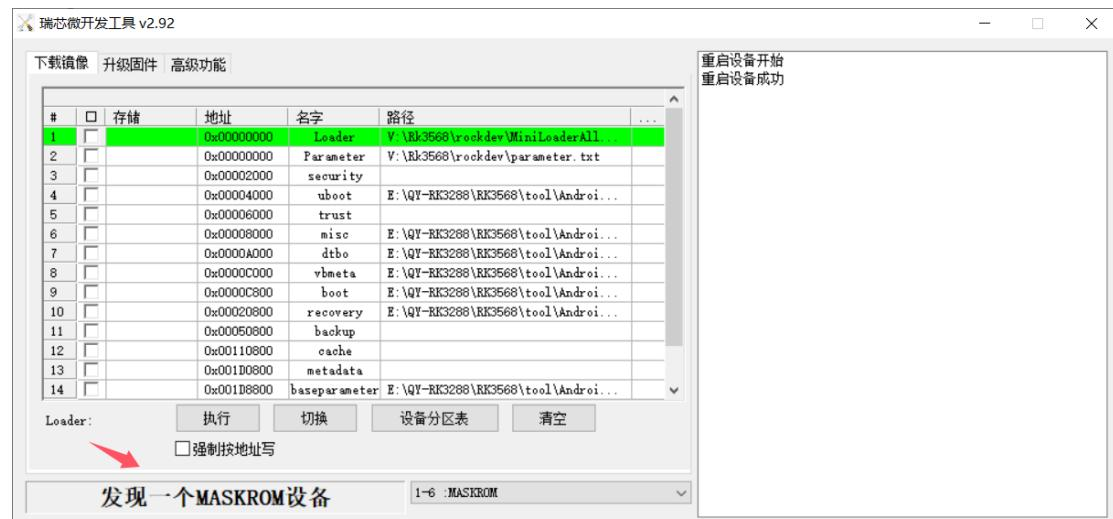
**Loader Mode:** The SOM boots normally; When debugging the kernel, the full image or partition-specific image is burnt to enter this mode, the flashed software is shown as below:
