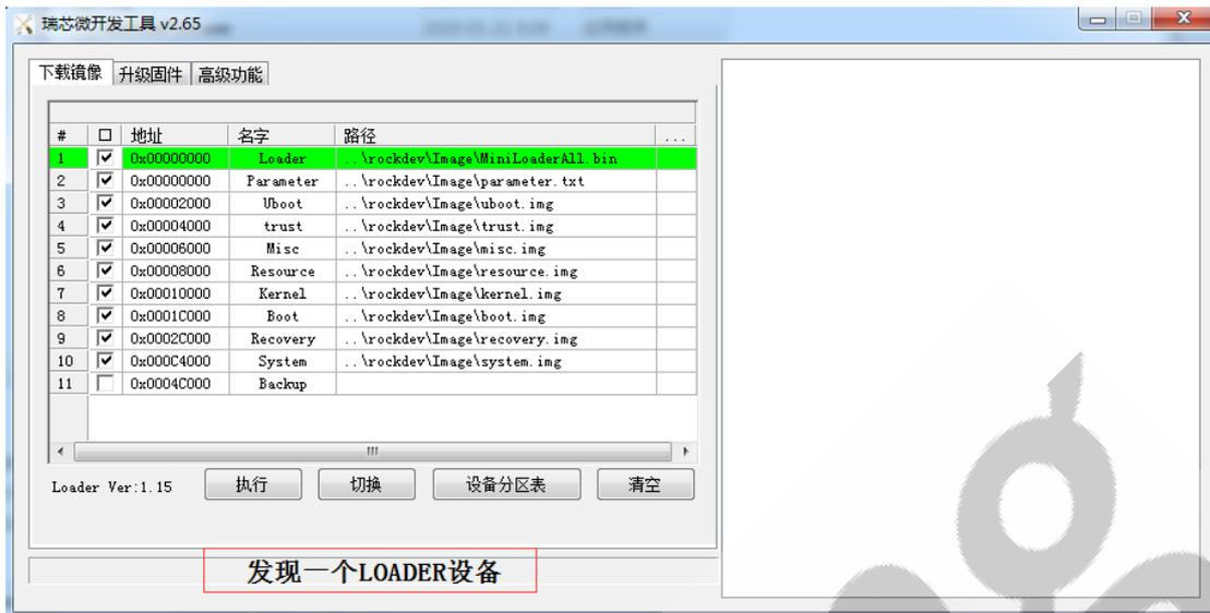
As above picture shown: a LOADER device is found, and image programming can be performed.
